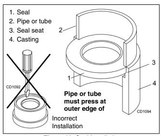
Figure 19. Seal Installation
